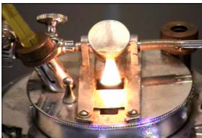
Figure 6: Closed Cup Outgassing – (Halogenated Hydrocarbon)
