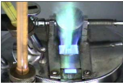
Figure 4 : Closed Cup Flash (Paraxylene)
