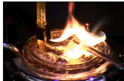
Figure 10 Open Cup Outgassing and Flash (Halogenated Hydrocarbon)
