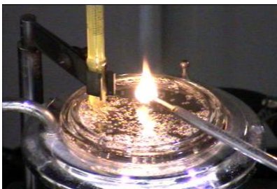
Figure 10 Open Cup Outgassing and Flash (Halogenated Hydrocarbon)
