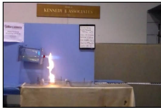
b) Flame front travel up the stream into vessel.
