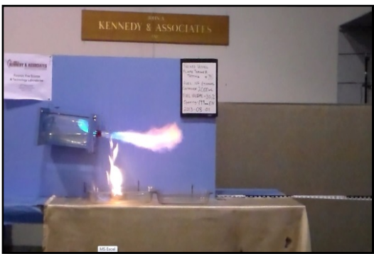
c) Vapor begins ejection as flame enters vessel.
