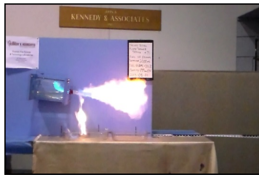
d) Liquid begins ejection as flame front progresses.
