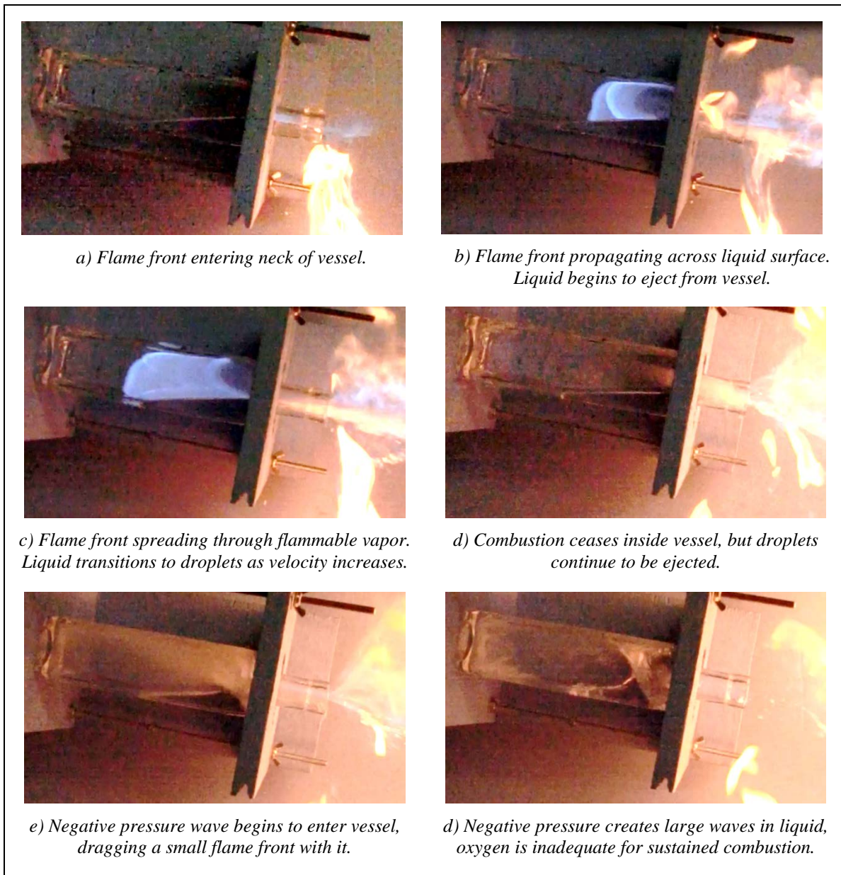
Figure 2. A series of still photos from digital high speed video. 500 ml square glass bottle, 16.4 mm ID opening x 50 mm neck, 20% filled, slow pour rate, opening not occluded.
